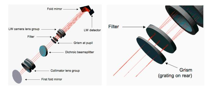
Figure 1. Optical layout of a NIRCam longwave (LW) channel with a grism. Left panel: Optical components are indicated, and light enters NIRCam from the first fold mirror at the bottom left. Right panel: Detail of the grism and filter region. Incoming light strikes the flat entrance face of the grism; its grating surface is on the rear side.
